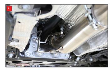
A/B) Re-fit all cables and hoses ensuring everything is clipped out the way and not near any moving parts.
